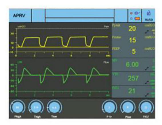
APRV is a time cycled pressure mode. In this mode, patient is allowed to breath spontaneously at two preset pressure levels. These are set using the Phigh and Plow controls. The maximum duration at each pressure during time cycling is set with the Thigh and Tlow controls.
