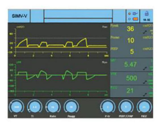
SIMV is a mixed ventilation mode that allows both mandatory and spontaneous breaths. The mandatory breaths can be volume-based (SIMV-V) or pressure-based (SIMV-P), and the spontaneous breaths can be pressure-assisted. Clinician can select pressure-triggering or flow-triggering in SIMV.
